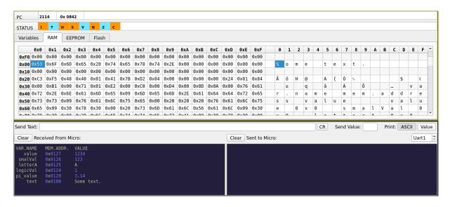
Figure 1: Table of values stroed in RAM memory of Arduino UNO controller.
